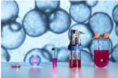
Figure 2 Various bioreactor systems for cultivating induced pluripotent stem cells (iPSCs) on microcarriers.
